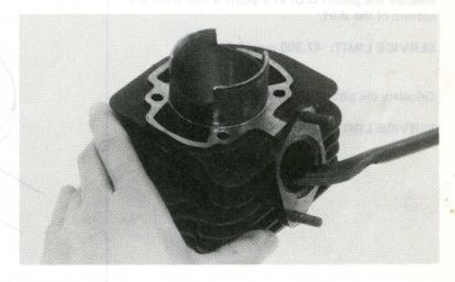
Inspect the cylinder bore for wear at three levels in X and Y directions. Use the largest measurement to determine the cylinder wear.
