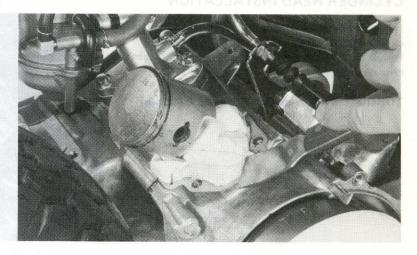
Place a new cylinder gasket on the crankcase.
