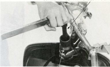
LOCK NUT WRENCH, 30 x 32 mm 07716-0020400 OR COMMERCIALLY AVAILABLE IN U.S.A.
