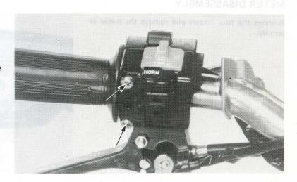
Remove the right handlebar switch by removing the two screws.
