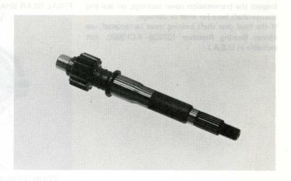
Inspect the countershaft and gear for wear or damage.
