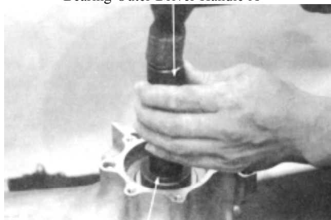
Bearing Outer Driver, 42x47mm Pilot, 20mm
