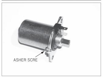
Align the front bracket with the cover. Tighten the washer screw.
