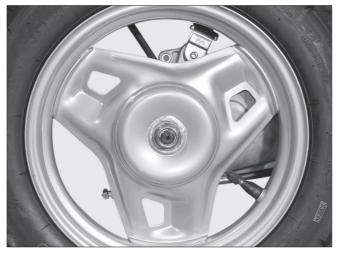
Insert the washer, and tighten with the U nut.
