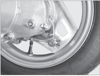
Install the brake arm joint B.
